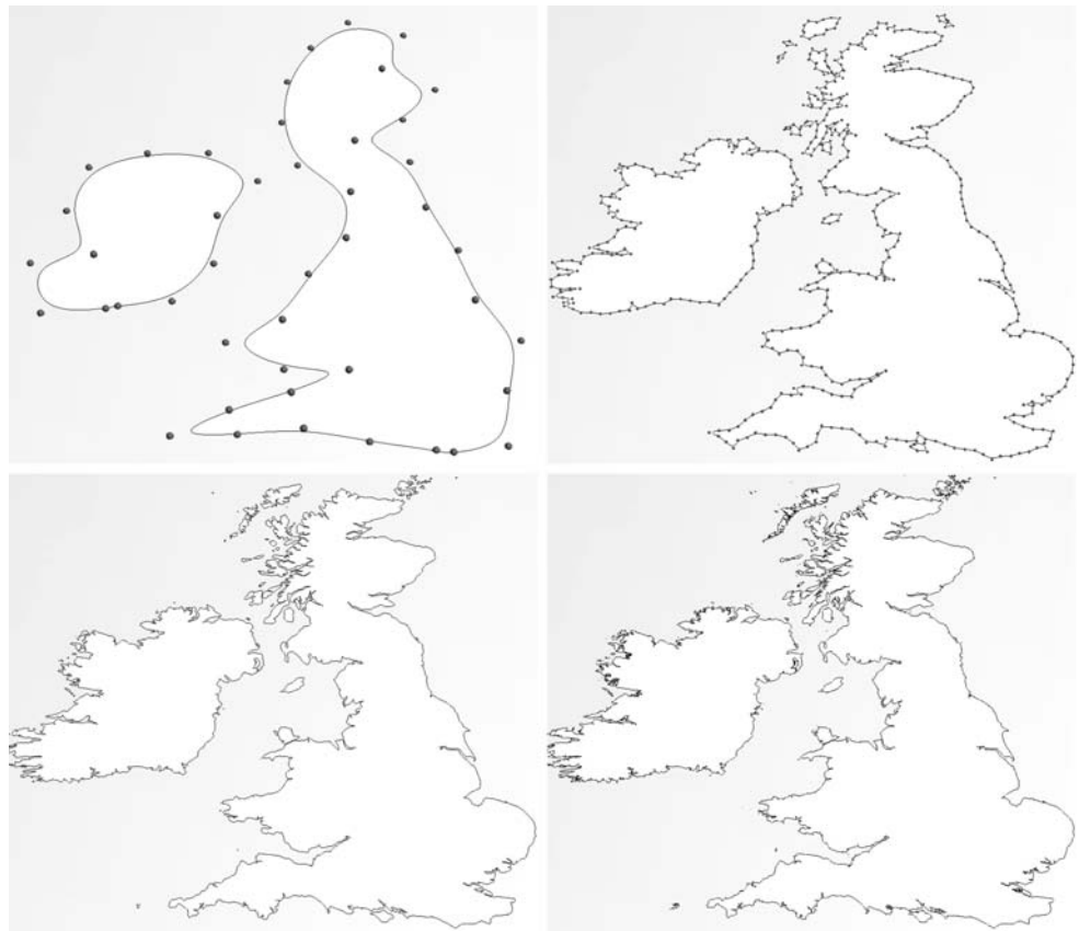
Fig. 5 Great Britain and Ireland with resolutions of 100 km ( top/left ), 15 km ( top/right ), 1.5 km ( bottom/left ), and 150 m ( bottom/right ). Splines control points are depicted on the geometry with the two lowest resolutions
